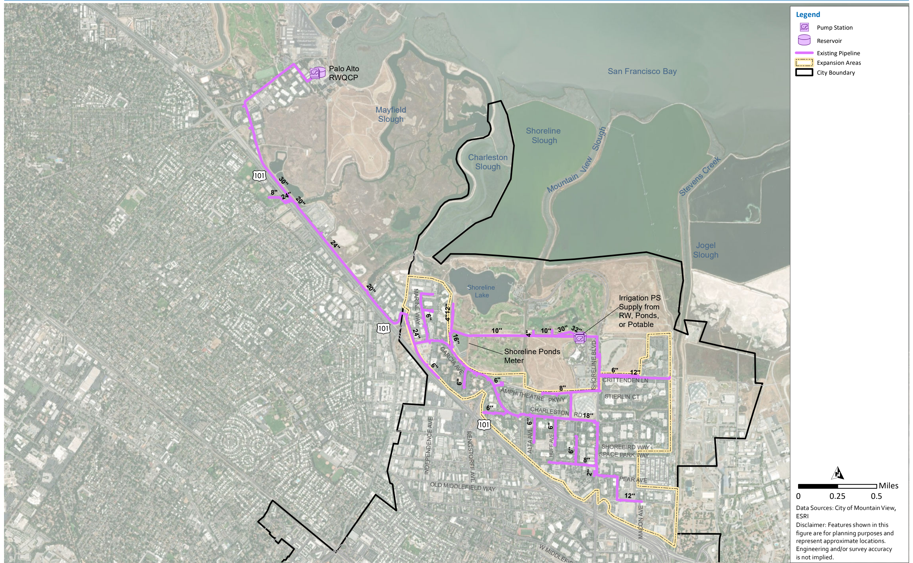
Figure 2.1 Existing Recycled Water Distribution System System
