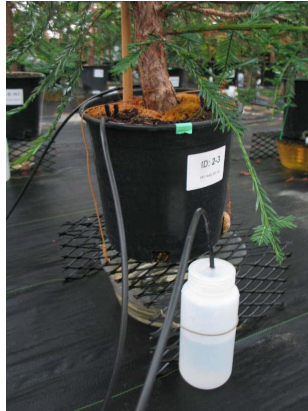
Figure 5. Saucer under pot stand for leachate collection and bottle for irrigation treatment collection.
