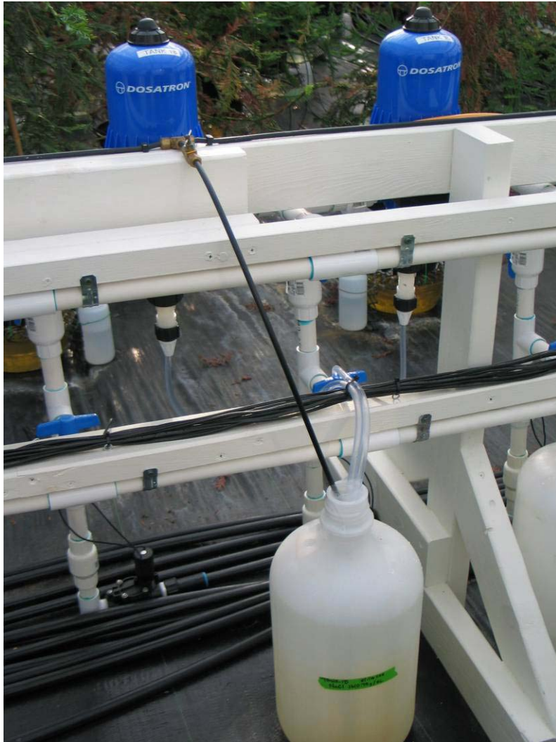
Figure 4. Eight liter concentrate bottle supplying two injectors. Concentrate solution was agitated by pressurized air delivered through 0.635 cm black tubing.
