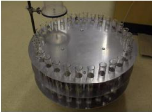
(a) A picture of one of three fraction collectors used in this experiment.
