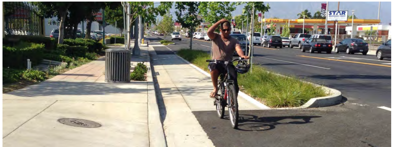
A one-way protected bicycle lane, such as this one in Temple City, is proposed for Shoreline Boulevard. Image from Joe Linton, Streetsblog.
