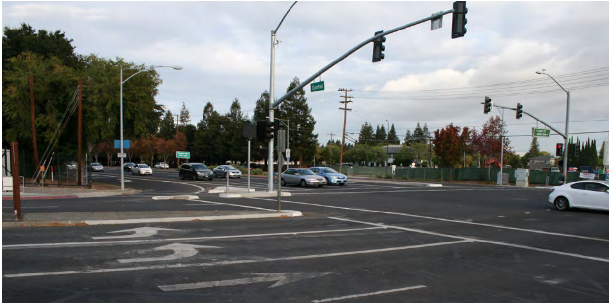
The existing configuration of Castro Street at Central Expressway creates challenges related to clearing of the Caltrain tracks and crossing time for pedestrians.
