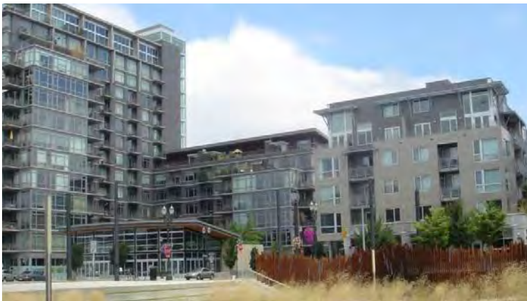
7e. Differentiate When multiple buildings are developed on a single block or parcel, each building should be differentiated through site design, building massing and design, and building materials and finishes.
