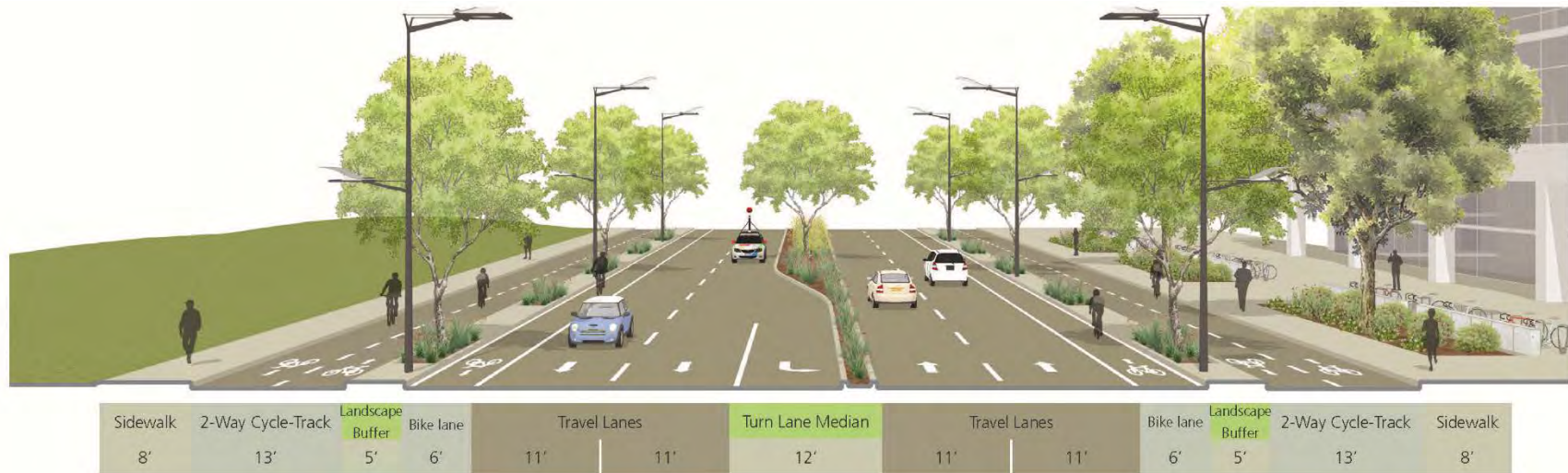
Figure 26: Gateway Boulevard: Potential Configuration of Amphitheatre Parkway
