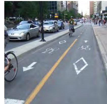
An example of a two-way cycle track with a buffer next to traffic.
