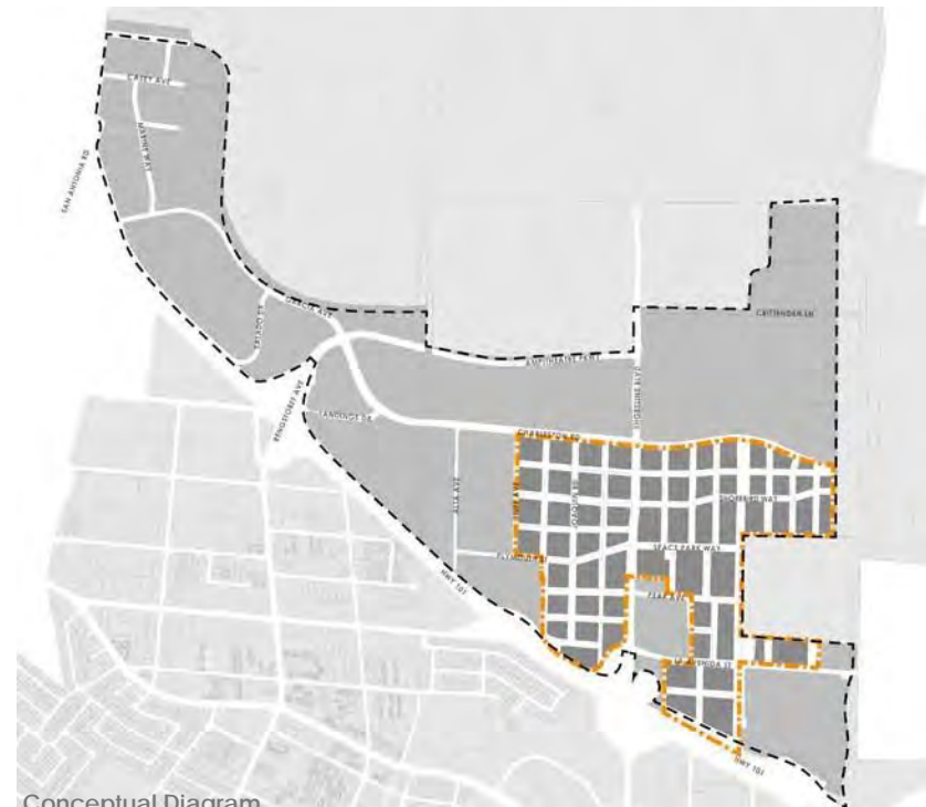
Conceptual Diagram 1b. Create small blocks sizes should be small enough to create allow frequent intersections and encourage walking and bicycling. Space Typically intersections should be spaced in general, at least every 400 feet.
