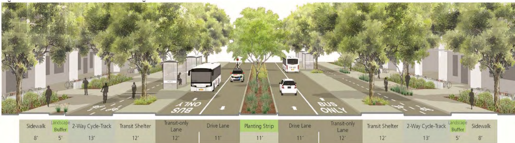
Figure 29: Transit Boulevard: Potential Configuration of Charleston Road
