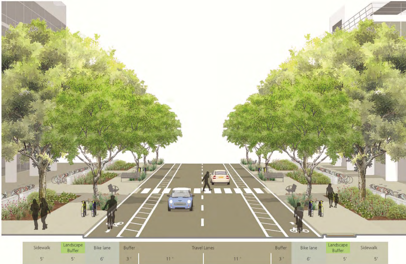
Figure 32: Access Street: Potential Cross Section
