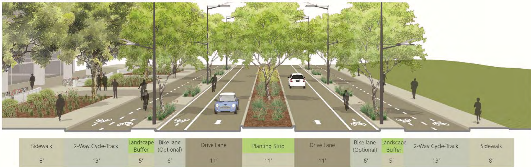
Figure 30: Transit Boulevard: Potential Configuration of Garcia Avenue
