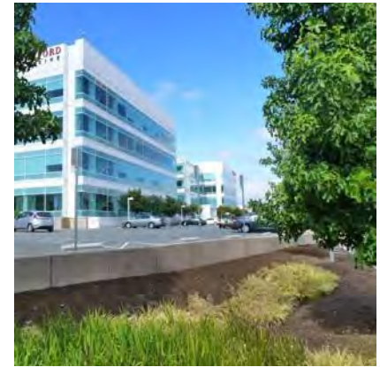
Bioswales adjacent to a surface parking lot.
