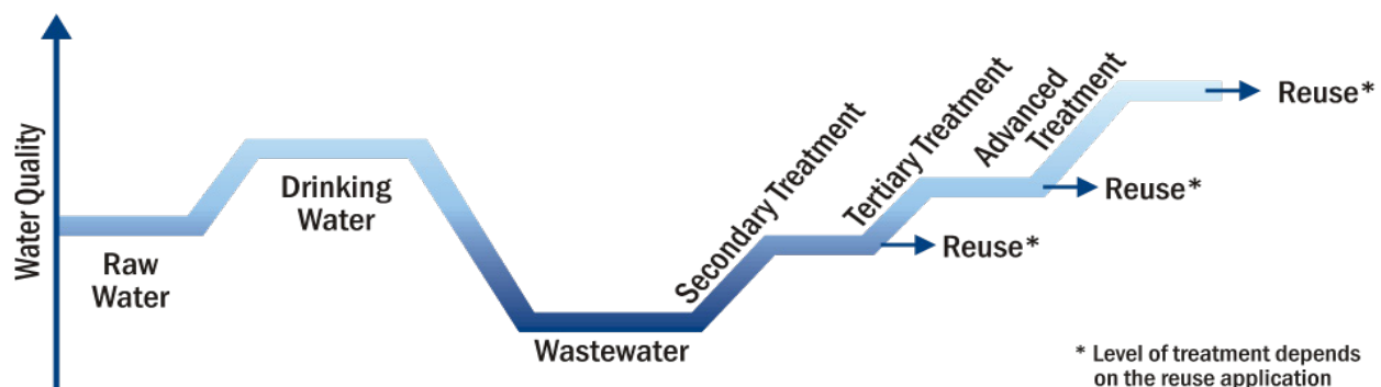
Figure 1-3 Treatment technologies are available to achieve any desired level of water quality
