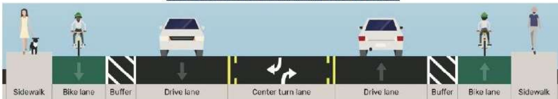
OPTION C: ROAD DIET OPTION - TWO-LANE SECTION WITH BUFFERED BIKE LANES (NO ACCESS RESTRICTION ON SIDE STREETS)
