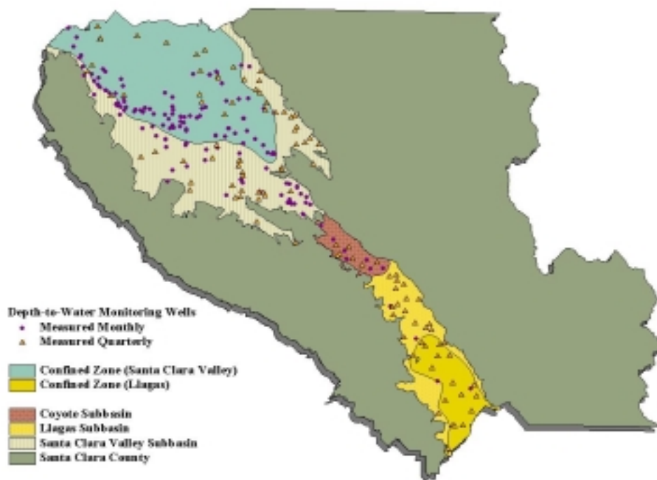
Figure 4-2 Groundwater Elevation Monitoring Wells
