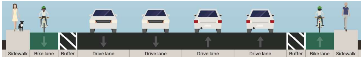
Figure 3: Typical Cross-Section—Alternative 1 (No Side Street Restriction)
