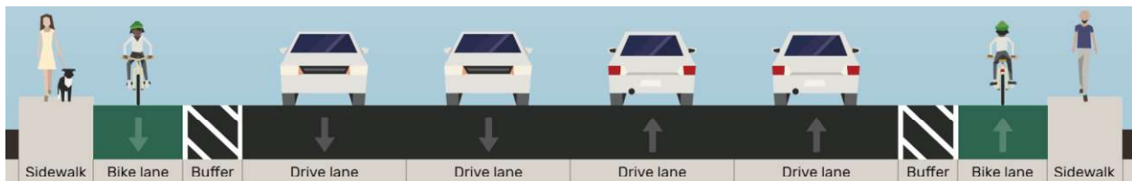
Figure 3: Typical Cross-Section—Alternative 1 (No Side Street Restriction)
