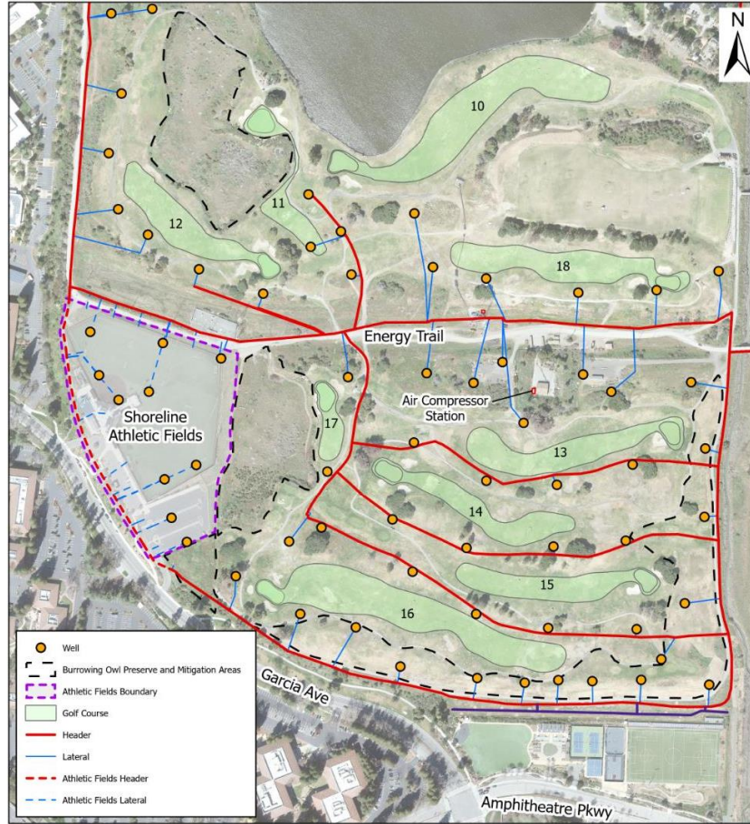
Figure 3: Back Nine Landfill Gas Collection and Control System (GCCS) and Golf Course (Holes 10 to 18)
